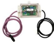
KC-2W N2K (NMEA2000) and NMEA0183 Bidirectional Converter
